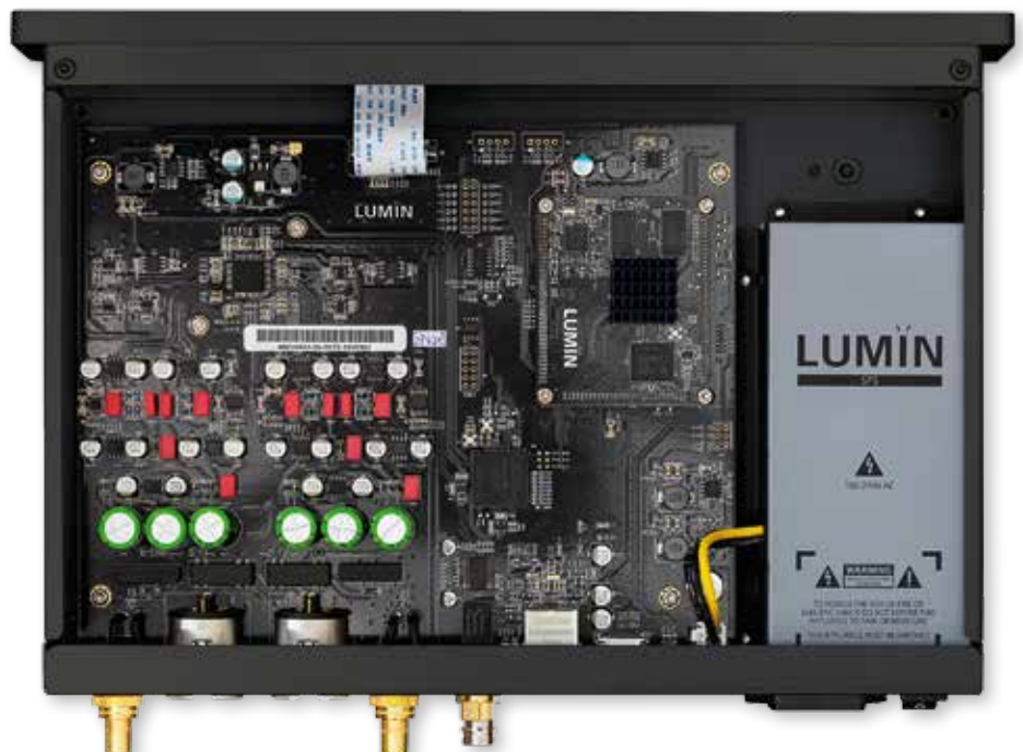
RIGHT: Fed from a screened PSU [far right] the D3's mainboard processor lies under a heatsink [centre right] with a Cyclone IV FPGA [bottom] and balanced analogue output board [bottom left] including an ES9028PRO DAC [top left]
