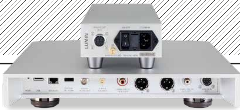
ABOVE: The Lumin X2 includes a USB-A host port for external drives, wired and optical Ethernet inputs (768kHz/32-bit; DSD512) alongside an S/PDIF output on BNC (192kHz/24-bit), and balanced/single-ended preamp outputs on XLR/RCA
